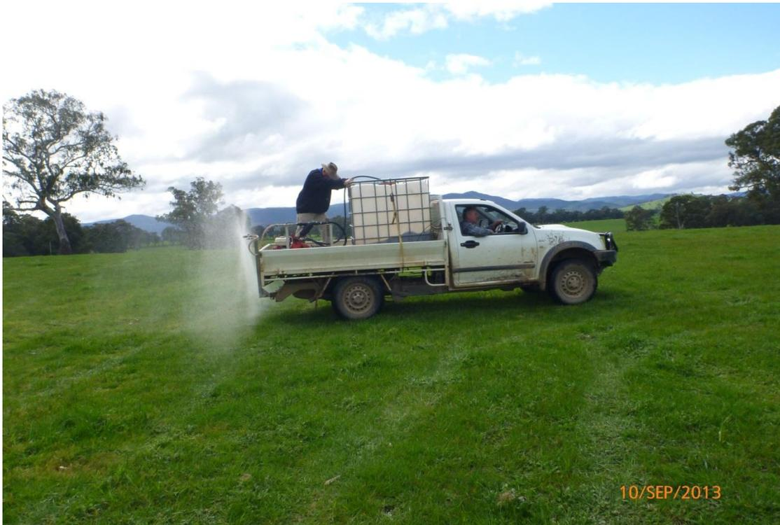
Use of bloat sprayer and fire pump to apply foliar sprays is much quicker and less hassle.
